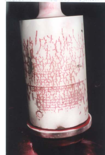
Fatigue cracking of valve cone
